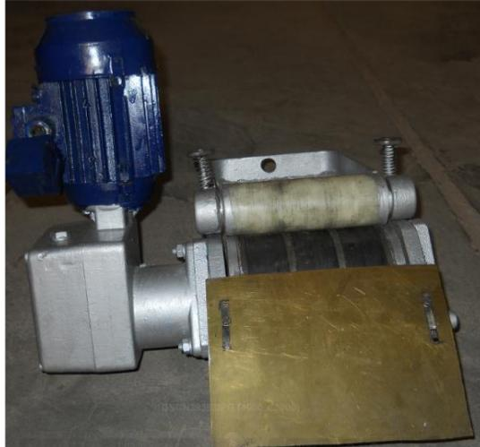
**FIGURE 2.** Front View of Magnetic Coolant Filter
