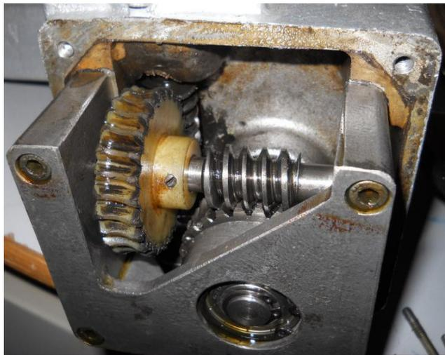
**FIGURE 3.** Double Reduction Worm Gear
