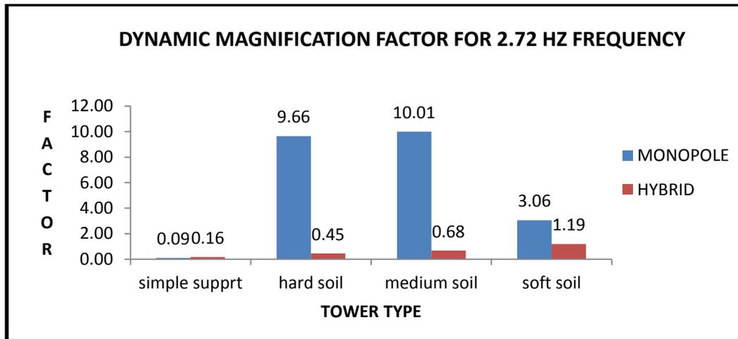
Figure 8. Comparison of DMF for 2.72 Hz Frequency
