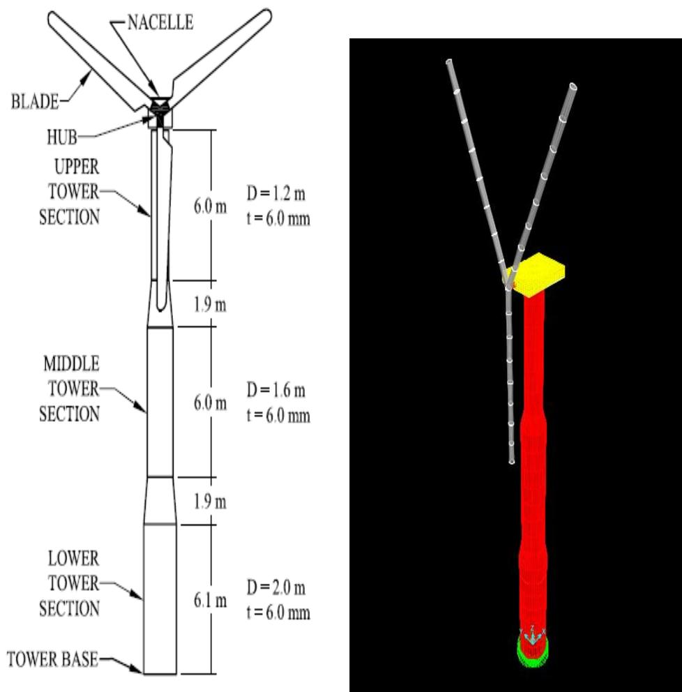
Figure 1. Dimensions of tower and its FEM model.
