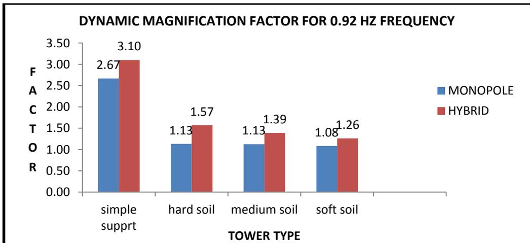
Figure 6. Comparison of DMF for 0.92 Hz Frequency
