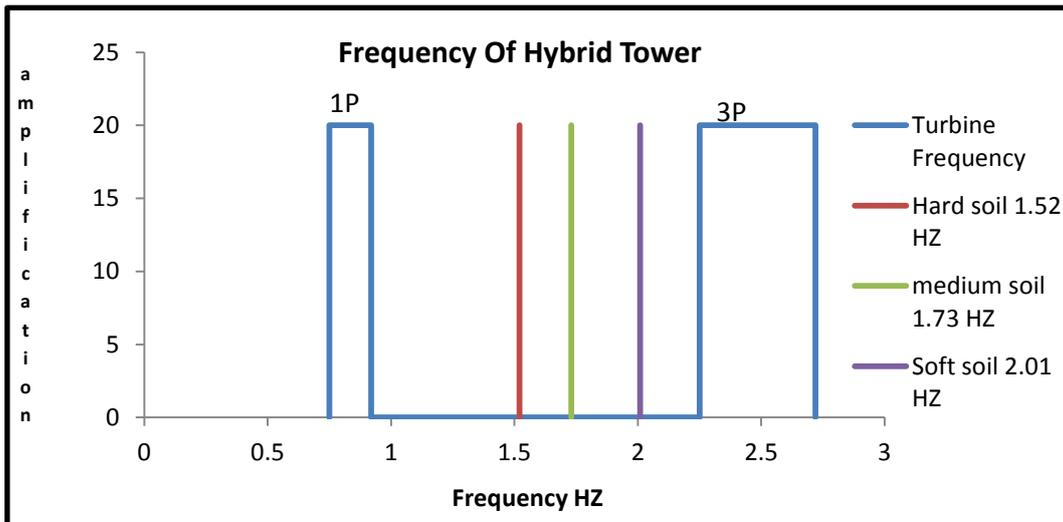
Figure 4. 1P and 3P Frequency of Hybrid Tower
