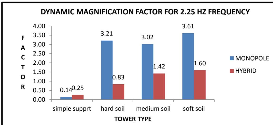
Figure 7. Comparison of DMF for 2.25 Hz Frequency
