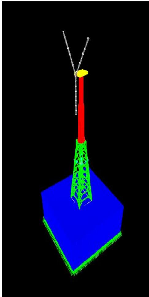
Figure 2. FEM model of hybrid tower with soil
