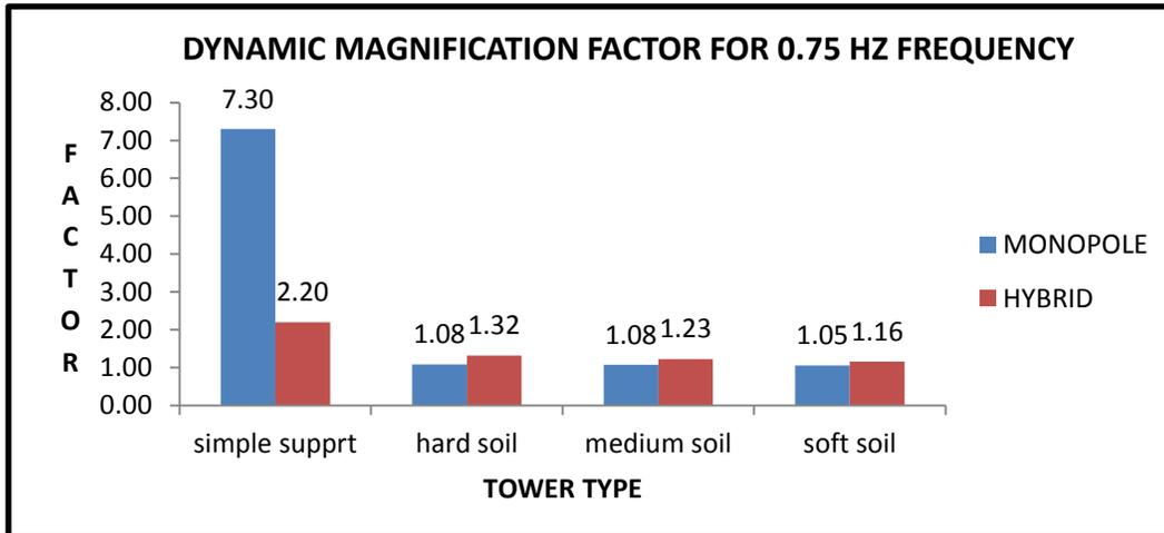
Figure 5. Comparison of DMF for 0.75 Hz Frequency
