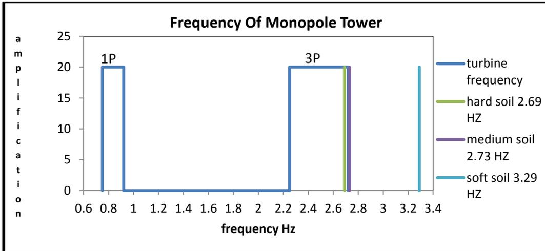
Figure 3. 1P and 3P Frequency of Monopole Tower
