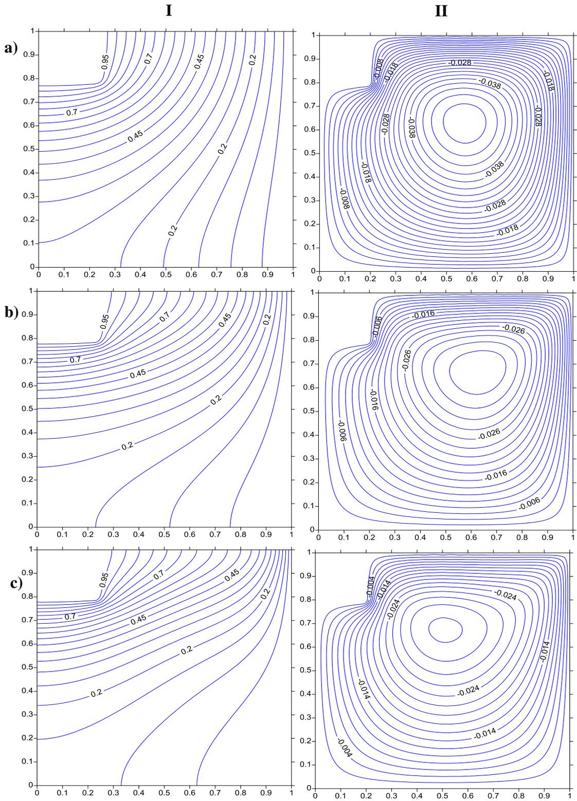
**FIGURE 3.** I) Isotherms II) Streamlines a)  $Ra = 10$  b)  $Ra = 50$  c)  $Ra = 100$  at  $R_d = 0.5$  and  $L_s = 0.2L$
