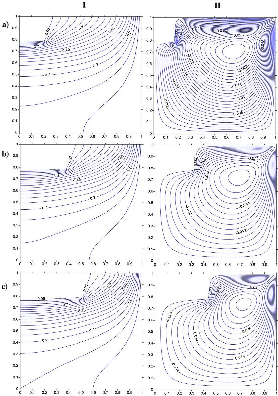
**FIGURE 2.** I) Isotherms II) Streamlines a)  $L_3=0.2L$  b)  $L_3=0.375L$  c)  $L_3=0.5L$  at  $R_d = 0.1$  and  $Ra = 100$
