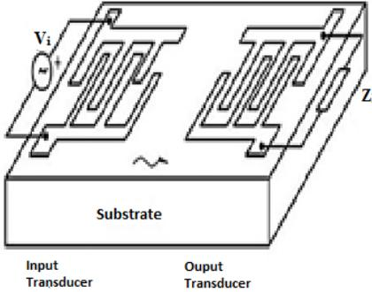
**FIGURE 1.** Basic Structure of SAW Gas Sensor
