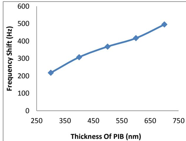
**FIGURE 6.** Frequency Shift vs Thickness of PIB
