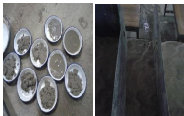
FIGURE 4. Samples collected for the calculation of moisture content
