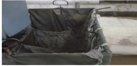
FIGURE 5. Sand trap/collector used to collect sediment water mixture for each run
