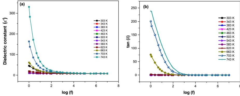
**Fig. 3(a) Variation of real part of dielectric constant  $\epsilon'$  and (b) loss tangent  $\tan \delta$  with frequency and temperatures for  $GdAlO_3$**
