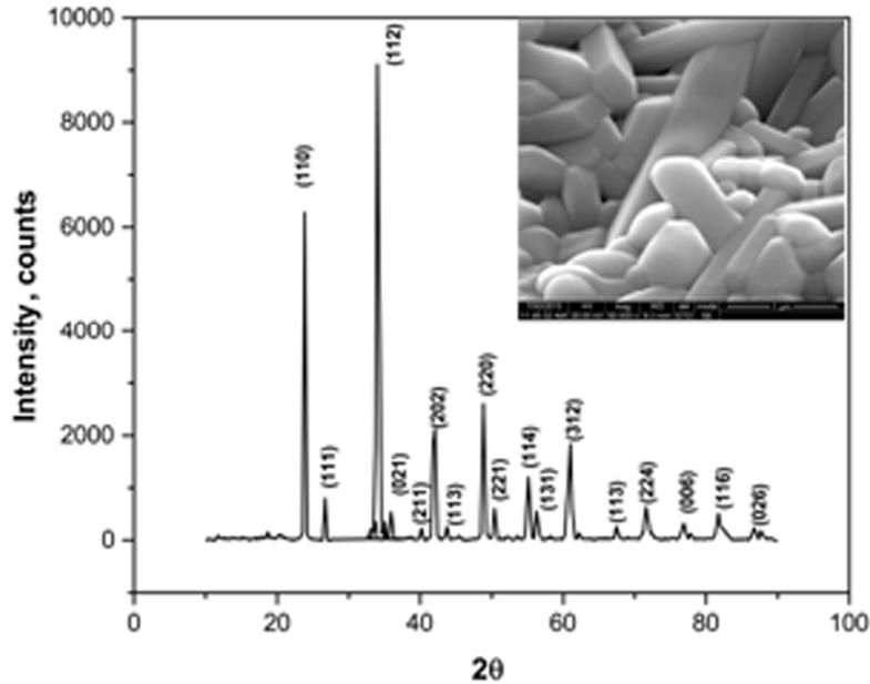
Fig. 1 XRD pattern of  $GdAlO_3$  sample calcinated at  $1000^\circ C$  for 2 h (inset shows HR-SEM image of sintered pellet )
