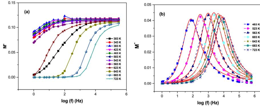
**Fig. 4(a) Real and (b) imaginary parts of electric modulus spectra at different temperatures. Solid lines are the theoretical fit.**
