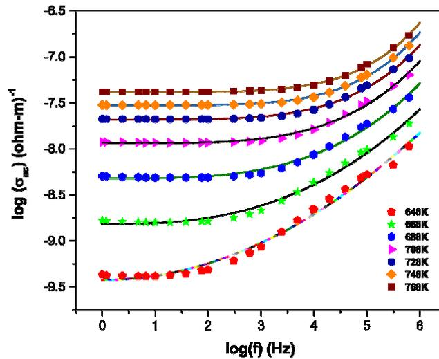
**Fig. 2** Frequency dependency of electrical conductivity at different temperatures. Solid lines are the theoretical fit.
