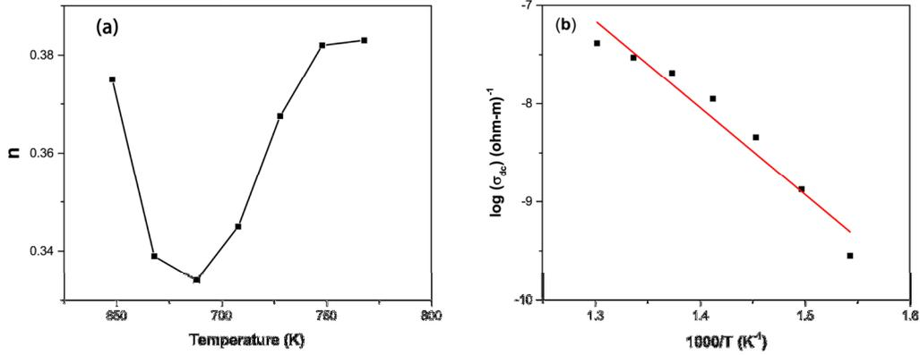
**Fig. 3(a) Variation of frequency exponent  $n$  with temperature and (b) Arrhenius plot for dc conductivity**
