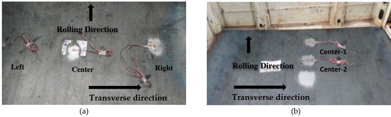
**FIGURE 1.** Installed strain gauge at- (a) The Head End, (b) The Tail end.
