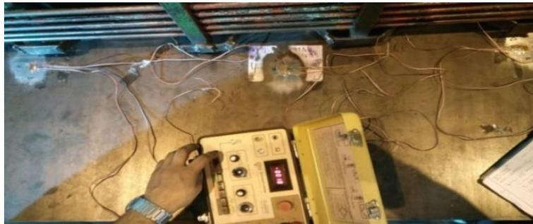
**FIGURE 4.** Strain measurement in steel strip after shear cut.
