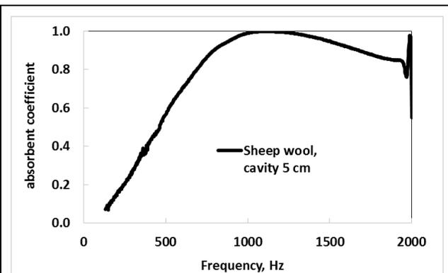
Figure 7. Sheep wool mounted at a distance of 5 cm from a back wall
