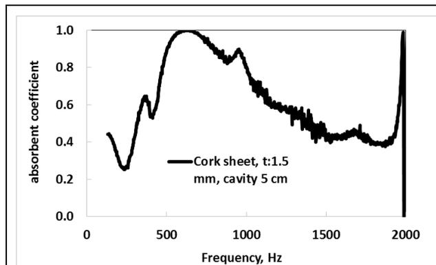
Figure 6. Cork mounted at a distance of 5 cm from a back wall
