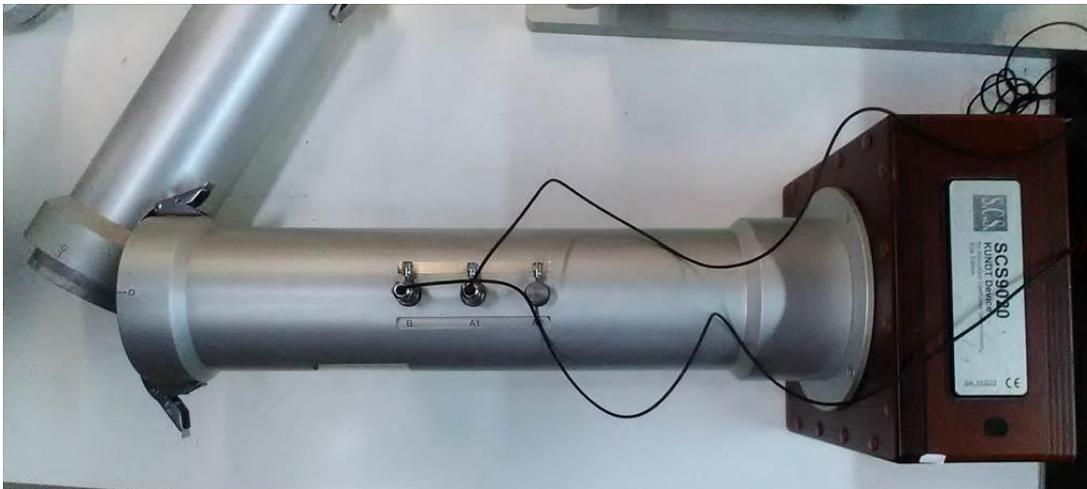
**Figure 1.** Impedance tube for the normal sound absorption coefficient measurement.
