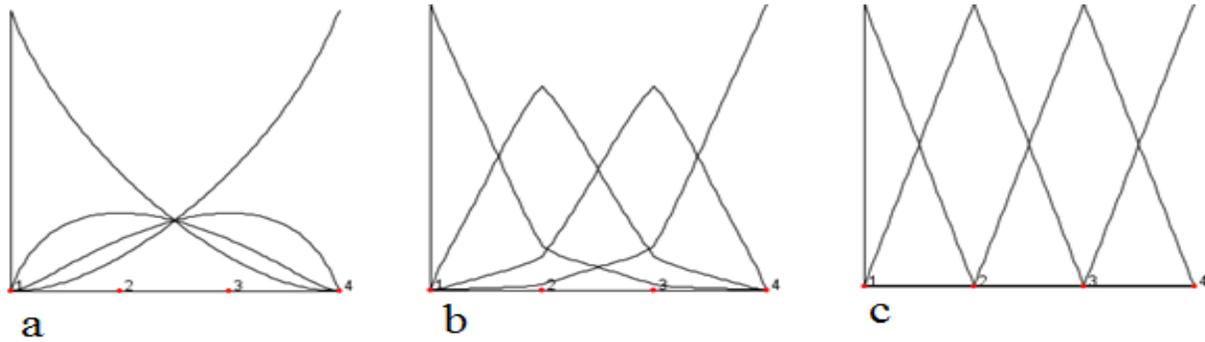
**FIGURE 5.** One dimensional Max-Ent basis functions with Gaussian prior for (a)  $\gamma=0.8$  (b)  $\gamma=2$  and (c)  $\gamma=4$
