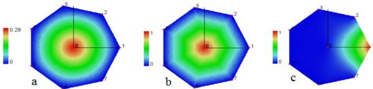
**FIGURE 3.**Two dimensional Max-Ent basis functions: (a) For interior node,  $\gamma=1.8$  (b) For interior node,  $\gamma=3.8$  (c) For boundary node
