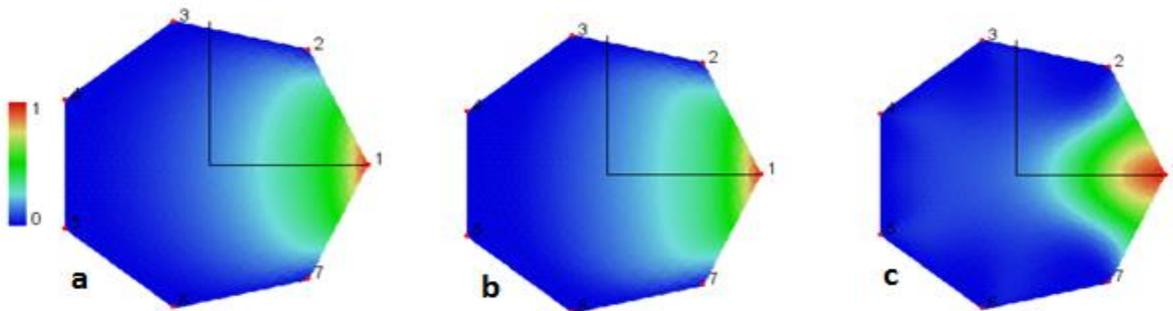
**FIGURE 6.** Two dimensional Max-Ent Basis functions for priors: (a) Constant (b) Cubic spline (c) Gaussian
