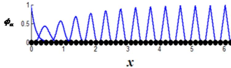
**FIGURE 1.**One dimensional example of seamless transition from meshless to finite elements achieved by tuning the value  $\gamma$ .
