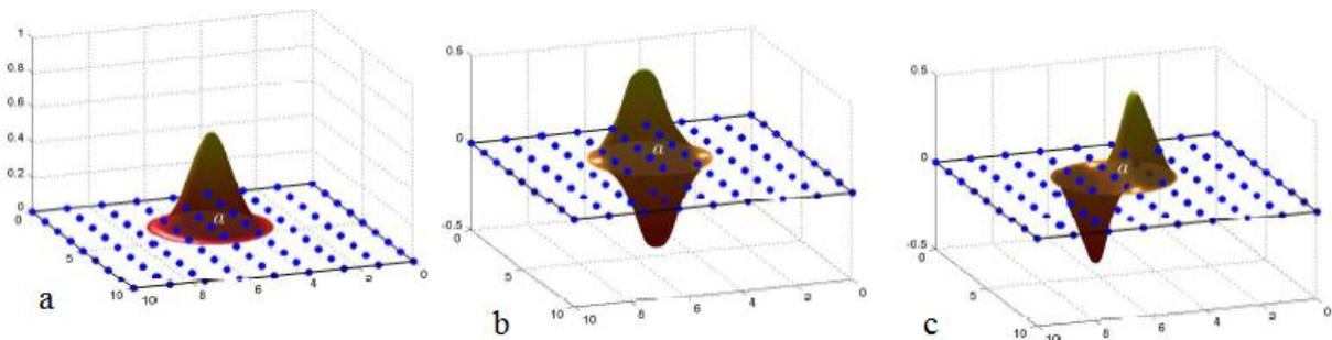
**FIGURE 9.**Two dimensional LME Basis functions for Quartic spline prior and derivatives for  $\gamma = 1.6$  [6]
