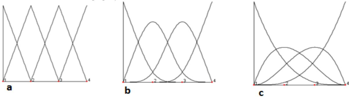
**FIGURE 4.** One dimensional Max-Ent basis with Compact cubic spline priors with (a)  $\gamma=4$  (b)  $\gamma=2$  and (c)  $\gamma=0.8$
