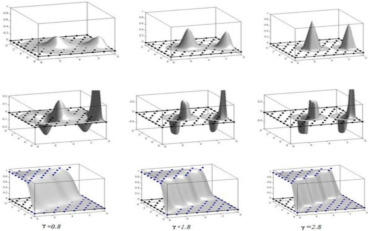
**FIGURE 8.**Two dimensional LME Basis functions for Gaussian prior  $\phi$  (first row) and derivatives  $\phi_{,x}$  (second row) and  $\phi_{,y}$  (third row) for different values of  $\gamma$
