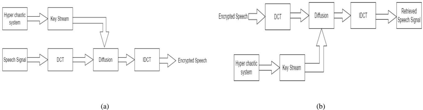
Fig.9 Block diagram of Secure Communication : (a) Encryption of speech Signal using Hyper chaotic system (b) Decryption of speech Signal using Hyper chaotic system
