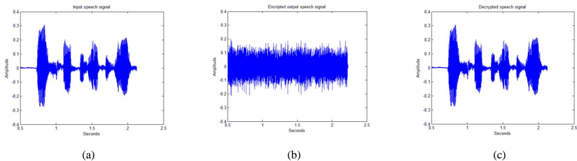
Fig.10 Encryption and Decryption using Hyperchaotic system : (a)Speech input (b)Encrypted Data (c)Decrypted Data
