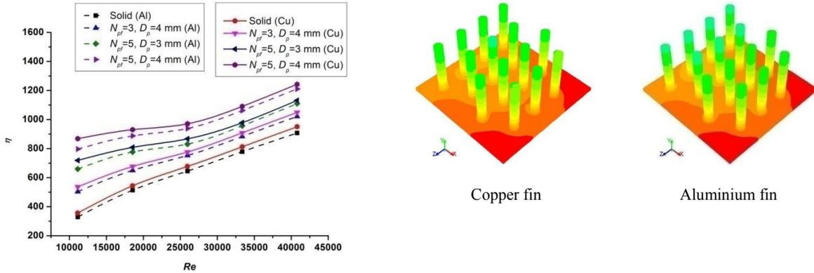
**FIGURE 3.** Effect of perforation on system performance ( $\eta$ ) for Al and Cu fin with  $N_{pf} = 5$ ,  $D_p = 3$  mm
