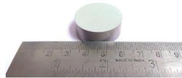
**FIGURE 5.** Specimen after sintering
