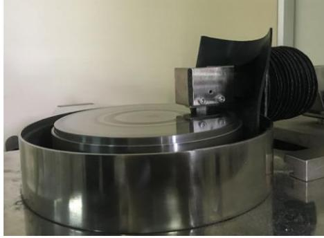
**FIGURE 6.** Pin-on-disc wear testing
