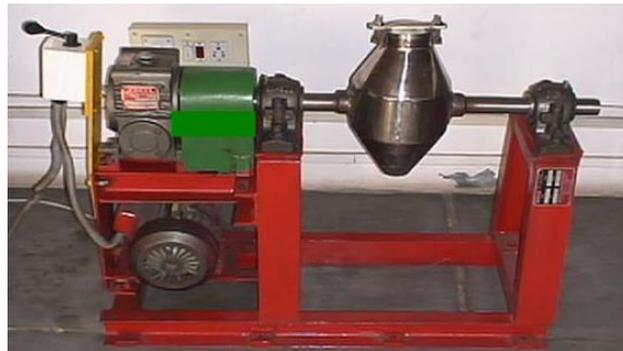
FIGURE 1.double cone powder mixer
