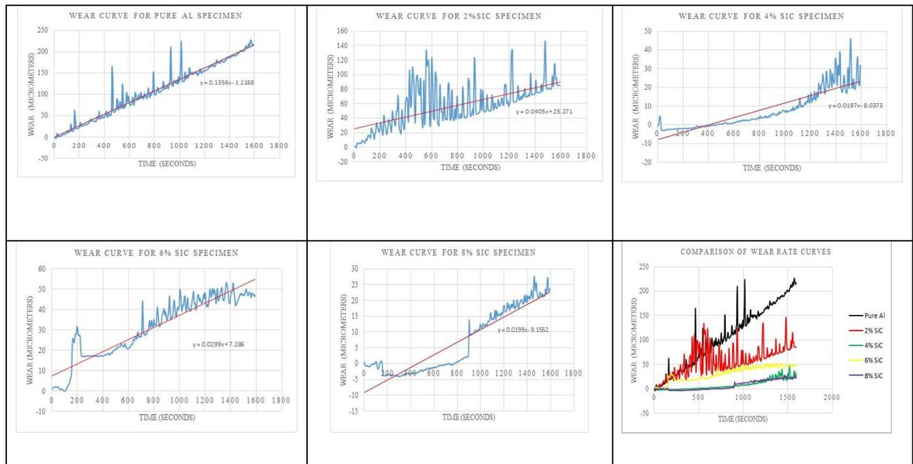
**FIGURE 8.** (a) Wear test for Pure Al (b) Wear test for 2% SiC + 4% Ni (c) Wear test for 4% SiC + 4% Ni (d) Wear test for 6% SiC + 4% Ni (e) Wear test for 8% SiC + 4% Ni (f) Comparison of wear rate curves after sliding 5000 m
