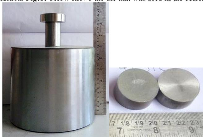
**FIGURE 2.** Die used for compaction **FIGURE 3.** Compacted green specimens
