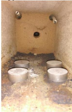
**FIGURE 4.** Specimen placed in muffle furnace for sintering
