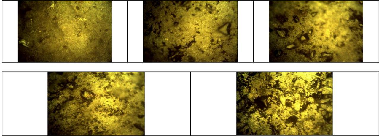
**FIGURE 10.** (a) Microstructure of Pure Al (b) Fig 4.17 Microstructure of 4% Ni and 2% SiC (c) Microstructure of 4% Ni and 4% SiC (d) Microstructure of 4% Ni and 6% SiC (e) Microstructure of 4% Ni and 8% SiC
