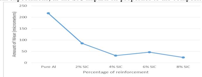
**FIGURE 9.** Comparison of amount of wear after sliding 5000 m
