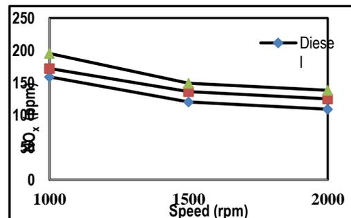
Figure 11: Variation of oxides of nitrogen with speed
