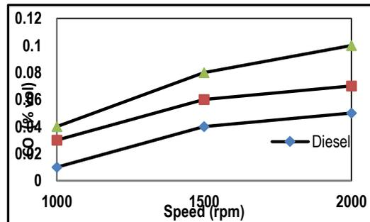
Figure 9: Variation of carbon monoxide with speed.
