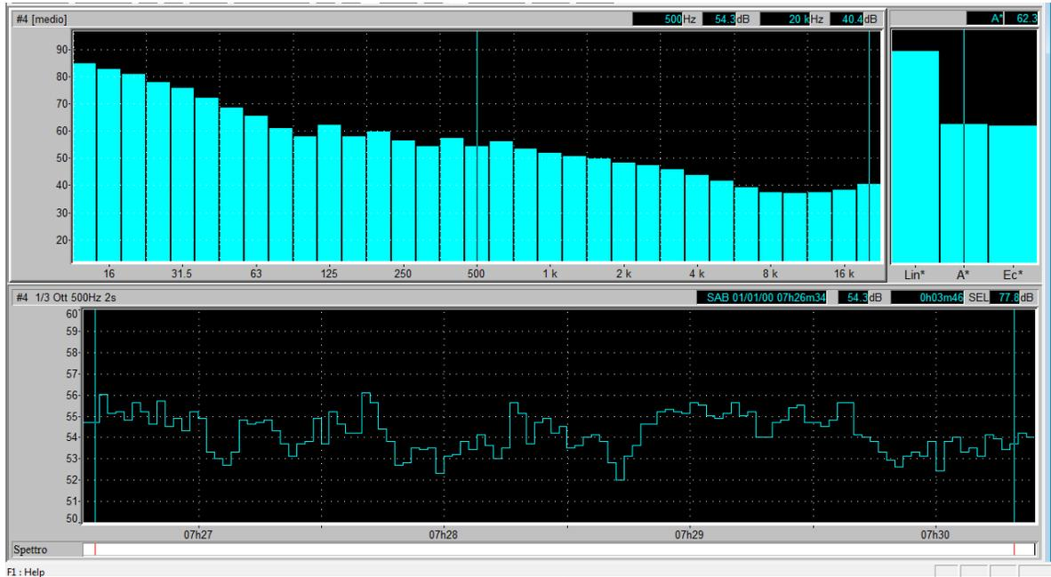
FIGURE 5. Frequency and time history for reticular towers at a distance of 30 m.
